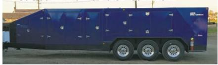
On board air compressor welder generator, tool storage, 4,500 Litre fuel, Transport Canada approved, 681 Litres of DEF fluid, electric fuel pump for use with on board generator or simply plug into 220 plug for quiet operation in farmyard by power station without starting motor. Many, many options are available on this unit!
